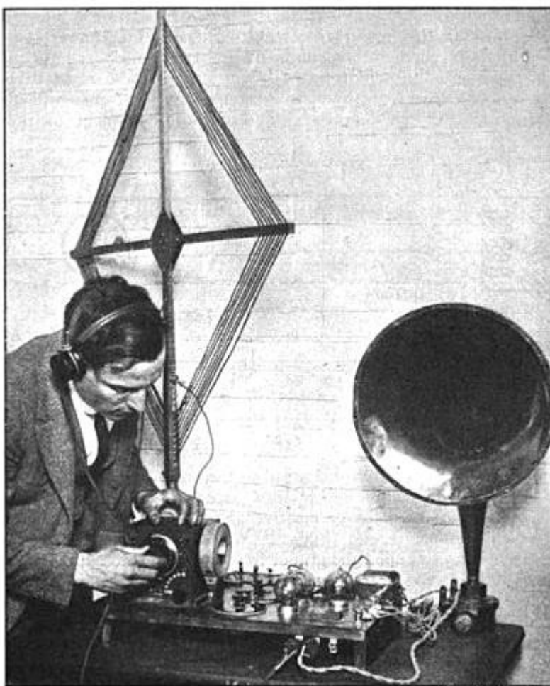
A THREE-TUBE SUPER-REGENERATIVE RECEIVING OUTFIT Used by E. H. Armstrong at the Radio Club of America's meeting held in Columbia University. Signals from a loud speaker were clearly heard over the entire auditorium
